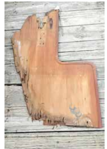
Yep, this was all that was holding up the starboard shroudline.
