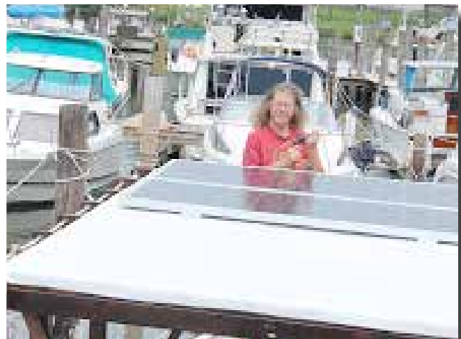
The much larger 325W panels being installed on Tesla's Revenge
