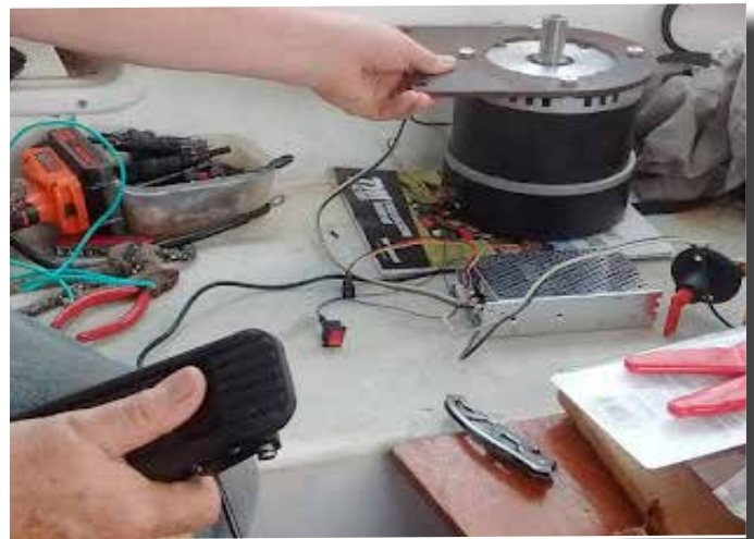
Power test of the 4.7 KW motor. Electric motors are torque heavy and far more compact than internal combustion engines. There will be more hurdles, we know that. The system is experimental and that means tinkering is a way of life. We are, however, sure of three things. 1) We wanted clean and quiet, tired of the racket and smell of internal combustion engines, 2) we wanted to live lightly on the earth, and most of all, 3) we want to be part of the future.
