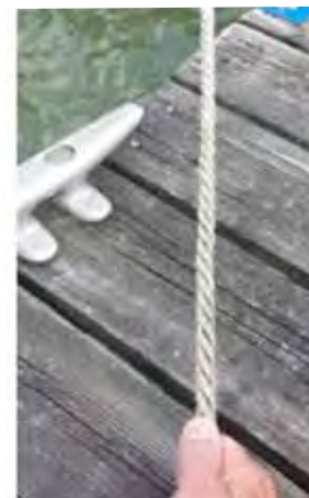
As the boat proceeds deeper into the slip, the dock line is off the cleat and the boat is not secure and continues deeper into the slip.
