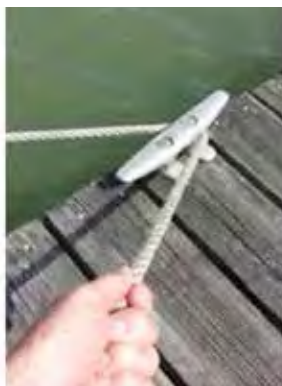
The boat's stern cleat is approaching from the left to the right. The son-in-law hooks the stern dock line underneath the "far horn" which is actually the "near horn" once the boat's transom passes the cleat.
